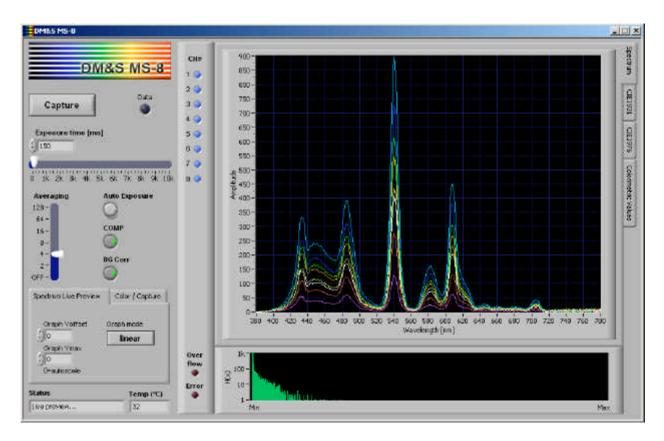
Control panel for setting of the parameters for the simultaneous acquisition of 8 spectra (0° - 70°), for display of the spectra and of the colorimetrc characteristics (CIE 1931, CIE 1976).
