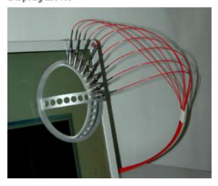
multichannel-measurig head with 8 collimators for viewing-directions from 0° to 70° inclination at constant azimuth
