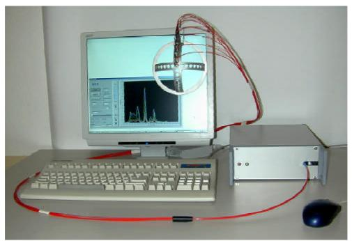
Experimental setup for demonstration of the principle of directional analysis of the emission of an LCD-monitor vs. viewing-direction.
